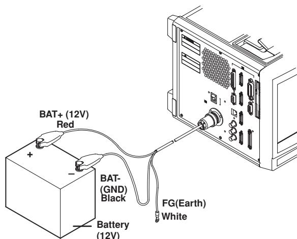
If you are creating your own DC power cord to match the specification for your environment, use the soldering-type connector that came with the package(1053JC).
